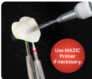
1. Sand blasting with 25-50µm alumina. Clean using ethanol, steam and ultra sonic cleaner. Dry sufficiently.
