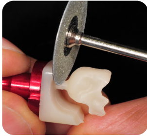
1. Removing sprue by diamond disc.
